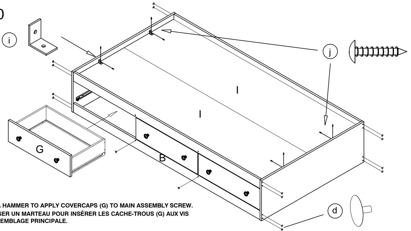
USE A HAMMER TO APPLY COVERCAPS (G) TO MAIN ASSEMBLY SCREW.
